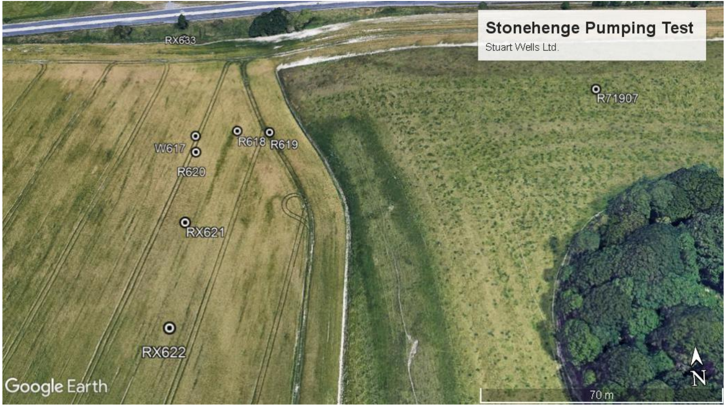
Figure 1: Pumping test well locations
